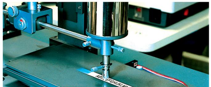
Abrasion resistant: after a 1kg sanding device was passed over the laminated labels 50 times, the text was unaffected
